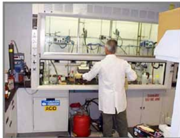
Figure 5.05 Hood with combination "A-style" sash.
